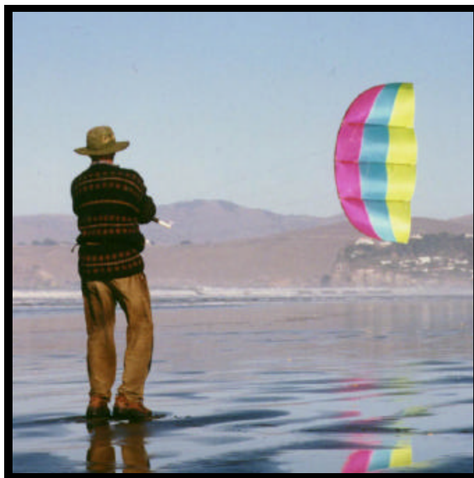
Peter Lynn testing a 3 spine, 2 meter square, C-Quad at Brighton Beach, Christchurch, New Zealand. April 1998 Photo by: Kane
